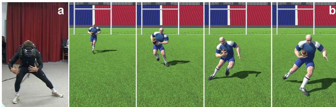
Figure 2.10. Example of the interaction in virtual reality between (a) a real defender, fitted with a VR headset, and (b) a virtual attacker who may or may not use a body swerve to go around him
